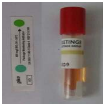
Fig 2. Chemical indicator strip (left) and Biological indicator vial (right) for EO sterilization process validation.
