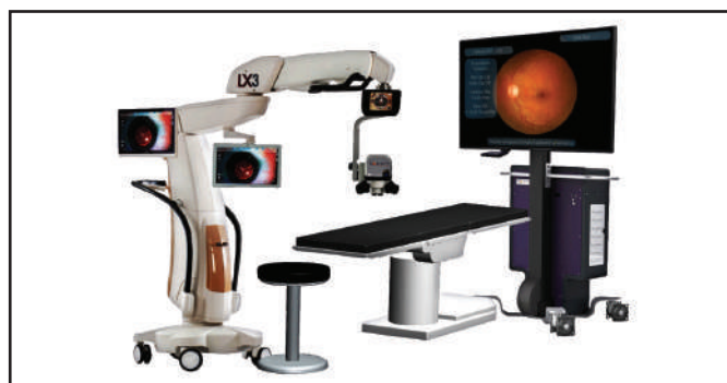
Figure 2: 3D Surgical display demonstrating microscope camera and high definition display (image provided by Novartis, NGENUITY® Media Release 21 ).
