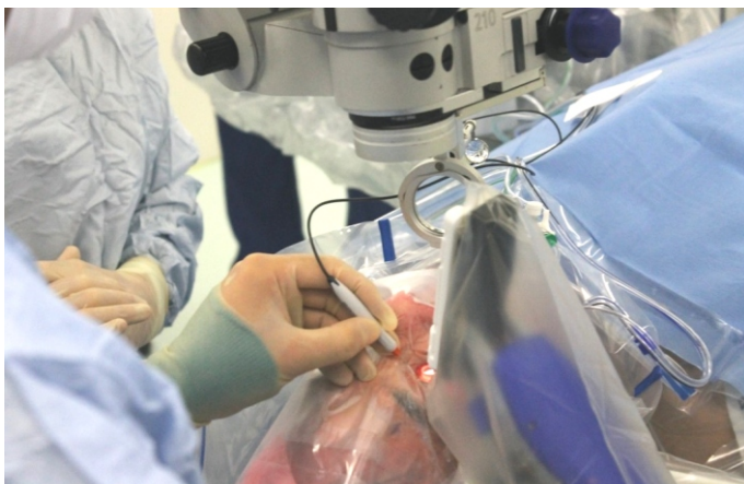
Figure 2 : The Preceyes robot affixed to the operating table in use during an internal limiting membrane peel procedure.
